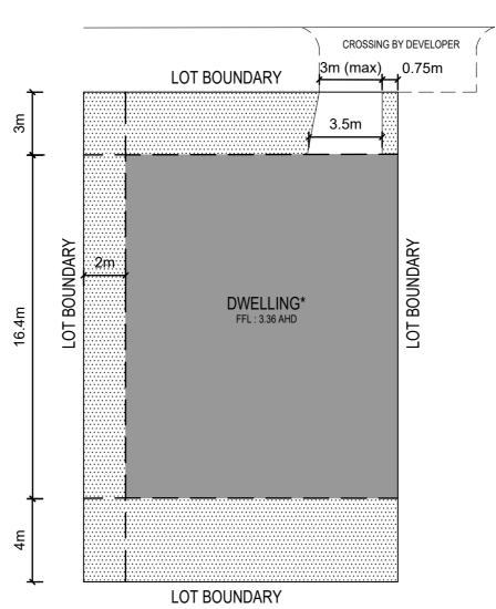
\* Maximum dwelling height 8.0m above minimum floor level of 3.36m AHD. Maximum garage height 4.2m above minimum floor level of 3.06m AHD
