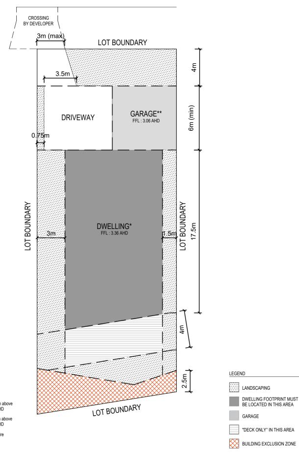
\*\* Maximum garage height 4.2m above minimum floor level of 3.06m AHD
