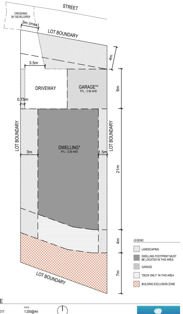
\*\* Maximum garage height 4.2m above minimum floor level of 3.06m AHD
