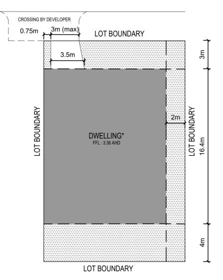
\* Maximum dwelling height 8.0m above minimum floor level of 3.36m AHD. Maximum garage height 4.2m above minimum floor level of 3.06m AHD For all BAL levels refer to Bushfire Management Plan Version 3 (31/01/2017) BUILDING ENVELOPE LOT 24 BROADBERACH INVERLOCH DATE SCALE JUNE.2017 SCALE JUNE.2017 SCALE JUNE.2017 SCALE JUNE.2017 SCALE JUNE.2017 SCALE JUNE.2017
