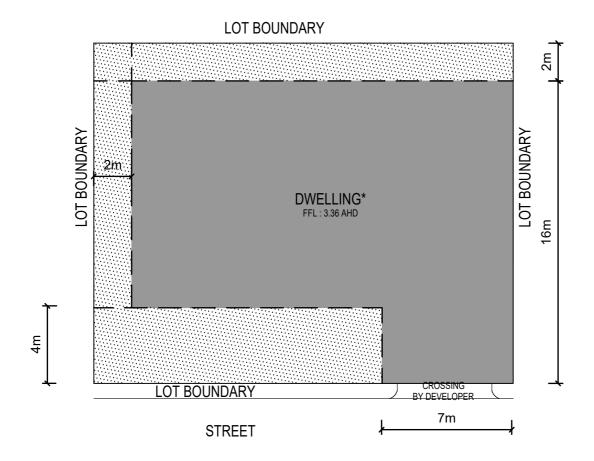
\*\* Maximum garage height 4.2m above minimum floor level of 3.06m AHD
