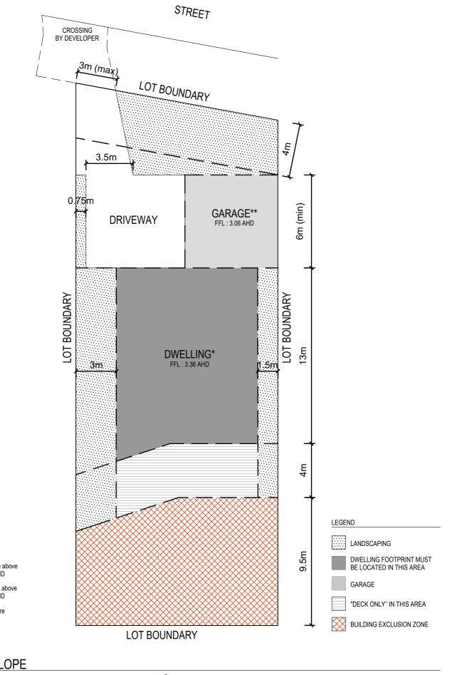
\*\* Maximum garage height 4.2m above minimum floor level of 3.06m AHD
