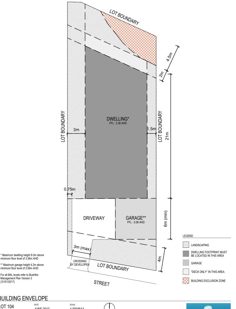
\*\* Maximum garage height 4.2m above minimum floor level of 3.06m AHD
